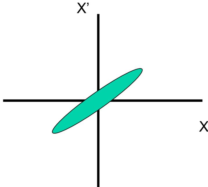
In a system where all the forces acting on the particles are linear (i.e., proportional to the particle's displacement  $x$  from the beam axis), it is useful to assume an elliptical shape for the area occupied by the beam in  $x$ - $x'$  trace space.
