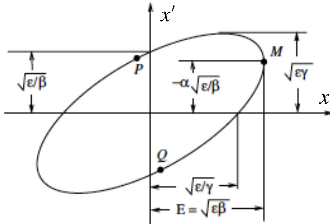
The slope of the beam envelope at point M:  $E' = \frac{\beta'}{2} \sqrt{\frac{\epsilon}{\beta}}$
