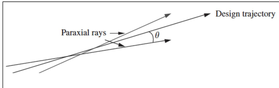
In a locally Cartesian coordinate system, we take the distance along the design trajectory to be  $z$ . The horizontal offset is designated by  $x$  and the horizontal angle is  $\theta_x$ .
