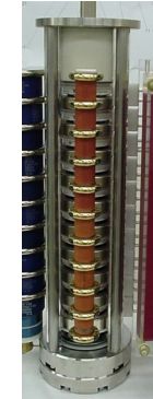
Stack of high-power semiconductor switches (GTOs)
