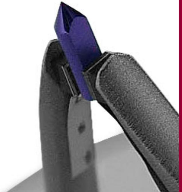
FEI **Mini Vogel Mount (MVM)** cathodes provide stable, high-brightness, long-lifetime operation for all major electron beam instruments. View FEI's standard parts for all major electron beam instruments in use worldwide on our [Applications Chart](#).
