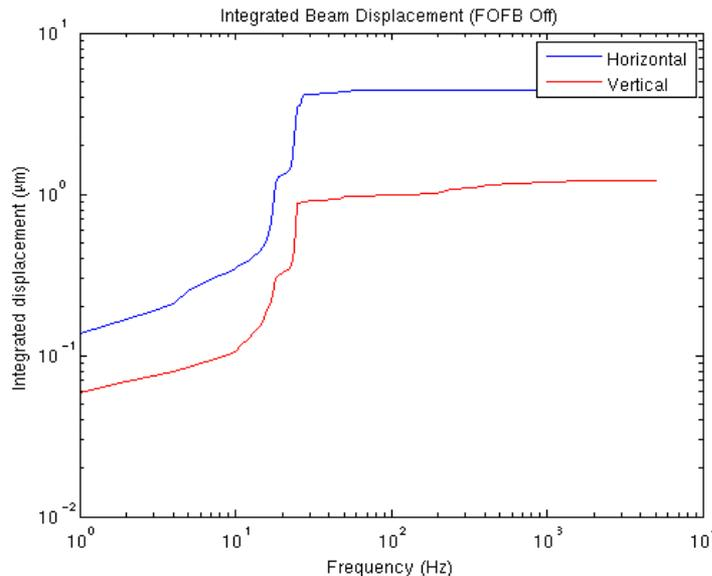
Horizontal and vertical electron beam displacement power spectral density (left) and corresponding integrated spectra (right) with the ‘fast orbit feed-back’ switched off.
