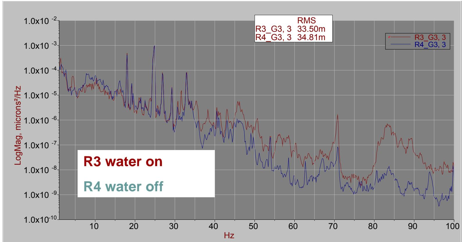
RMS (ie integrated) displacements – R3 is  $33.5 \times 10^{-9}$  m, R4 is  $34.8 \times 10^{-9}$  m
