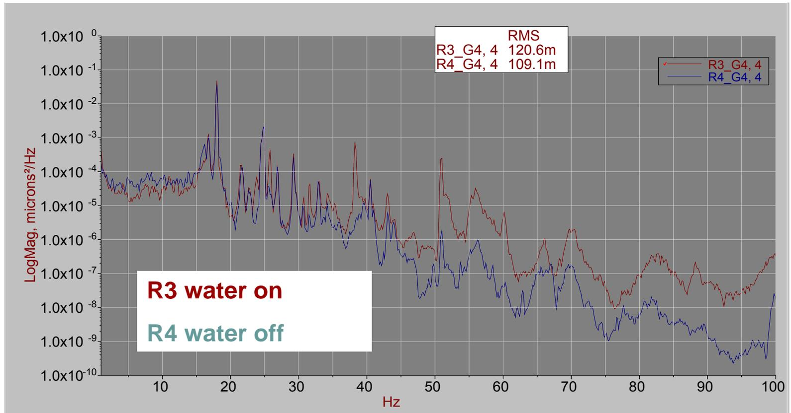
RMS (ie integrated) displacements – R3 is  $120 \times 10^{-9}$  m, R4 is  $109 \times 10^{-9}$  m
