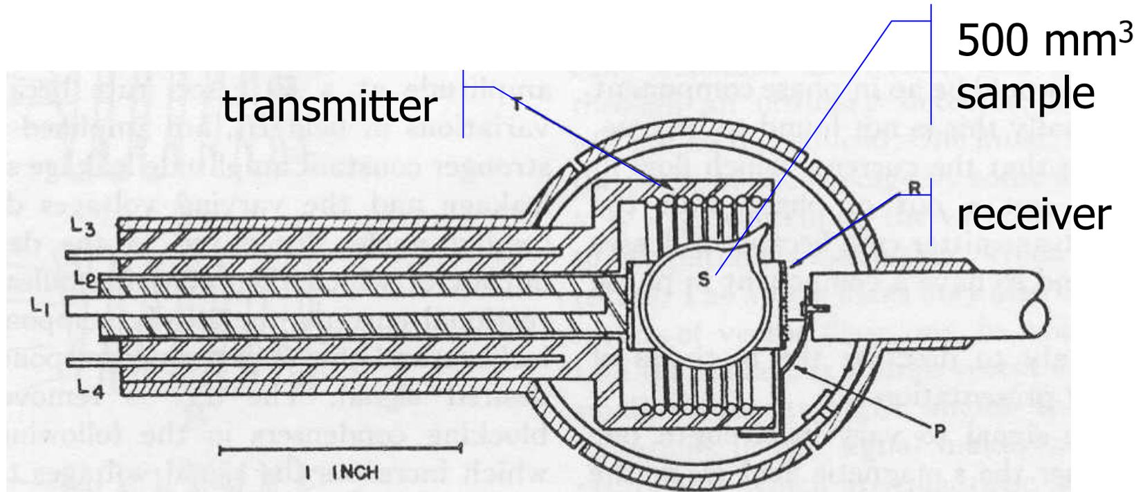
FIG. 4. Scale drawing of an *xy* section of the r-f head. The spherical sample *S* is surrounded by a receiver coil *R*, which is in turn surrounded by a transmitter coil *T*, the whole being encased in a shield. A rotably mounted paddle *P* is used to steer the transmitter flux. Leads to the receiver coil are the coaxial leads *L*<sub>1</sub>*L*<sub>2</sub> while the transmitter leads are *L*<sub>3</sub> and *L*<sub>4</sub>. The outer shield is split to avoid 60-cycle eddy currents.
