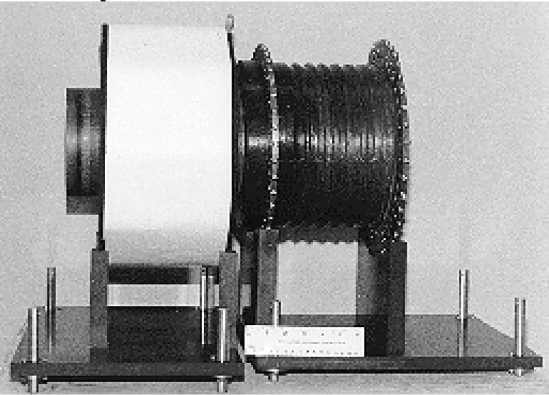
imploding flux compression generator (VNIIEF design)
