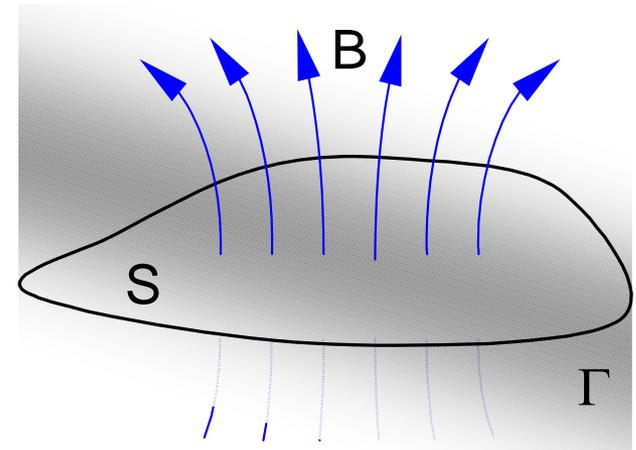
$$\varphi_{end} - \varphi_{start} = - \int_{t_{start}}^{t_{end}} V dt$$
