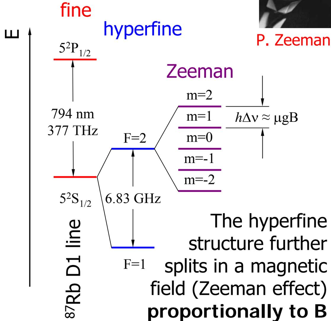
The hyperfine structure further splits in a magnetic field (Zeeman effect) **proportionally to B**
