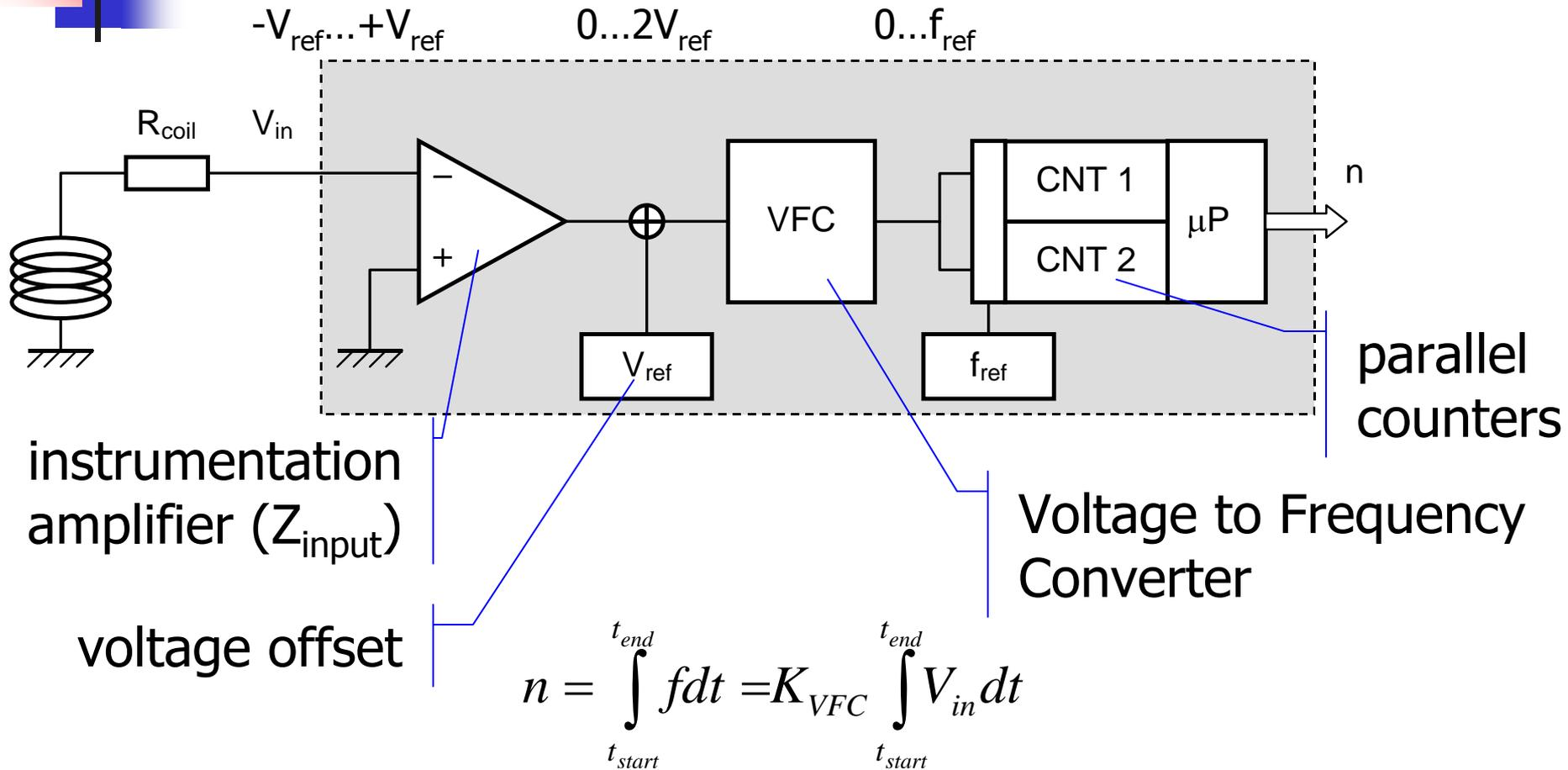
digital output, no cumulative error, 10...100 ppm accuracy !
