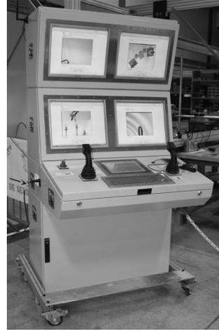
Viewing system with 4 pan tilt cameras. Control system with 2 joysticks installed behind shielding. Communication with WiFi over 100m
