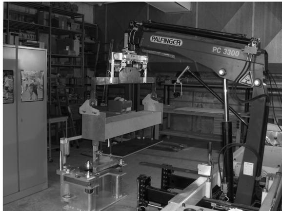
Dummy collimator installed on base using modified truck loader crane with camera viewing and remote control
