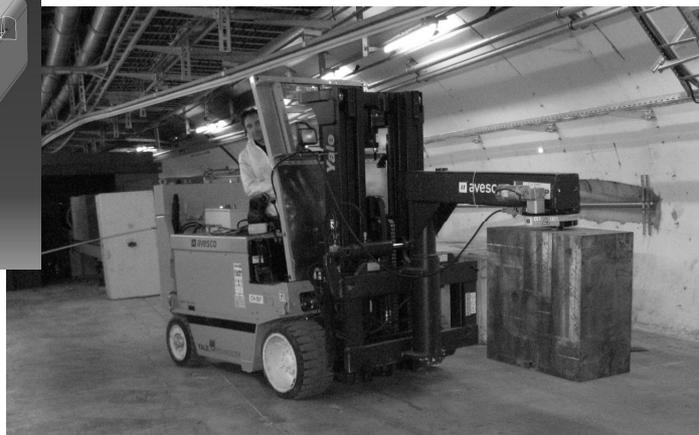
Fork lift equipped with powered rotation hook and operator shielding
