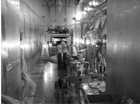
Most of the devices used during the dismantling process could be cleaned in the  $\beta$ - $\gamma$  box of ZWILAG and have been delivered back to PSI. The TC1 container is currently stored at ZWILAG and will be shipped to PSI in the 4<sup>th</sup> quarter of 2010 for decontamination (only the inner container is contaminated do to slight scraping of the AlMg3 safety hull during insertion).
