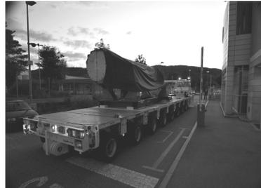
On July 6<sup>th</sup> the MEGAPIE target was transferred with a special transport container (TC1), fabricated by Skoda, from PSI to ZWILAG (Interim storage facility for nuclear power plant waste). Dose rate at surface of TC1 ~ 1  $\mu$ Sv/h. The transfer started at ~21:10 and took roughly 2 hours. Authorities (BAG/ENSI) were present and monitored the procedure.
