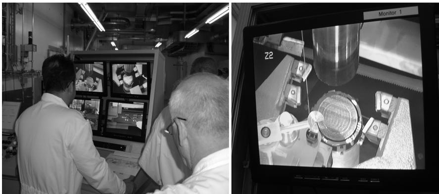
As the target had to be cut from bottom to top (hanging on a crane) the first cut was already one of the most important ones, the Beam Entrance Window.
