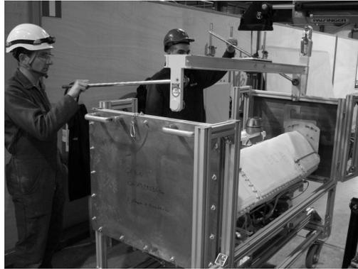
Shielded trailer for transfers (compatible with 1 tonne lift):
