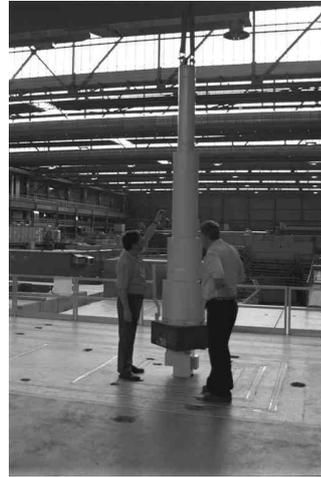
Exchange flasks are shielded „mini cranes“ that can be remote controlled – on a step by step basis - from a safe distance.
