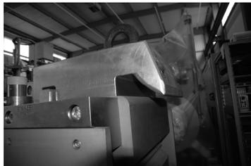
**Magnet is hung onto the vacuum chamber**
