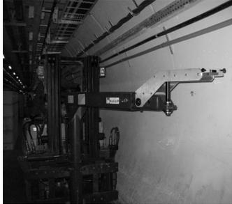
Reduced lost height tooling for lift truck boom
