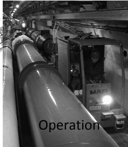
Remote controlled inspection vehicle for LHC
