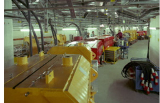
Dipole magnets (red), quadrupole magnets (yellow)
