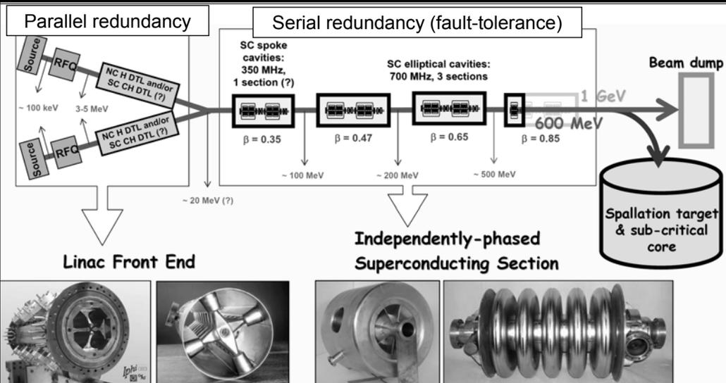
Modular & upgradeable concept – Maximized electrical efficiency – Optimized for reliability
