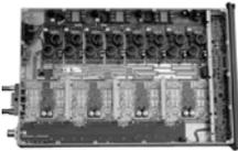
Figure 8 – HARRIS liquid cooled UHF transmitter<sup>30</sup>.
