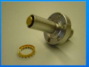
button electrode for use between the undulators of the TTF II SASE FEL (courtesy D. Noelle and M. Wendt, 2003)
