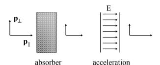
similar to radiation damping, but there is multiple scattering in the absorber that blows up the emittance
