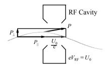
The transverse momentum, or the amplitude of the betatron oscillation remains small
