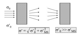
to minimize the blow up due to multiple scattering in the absorber we can **focus** the beam
