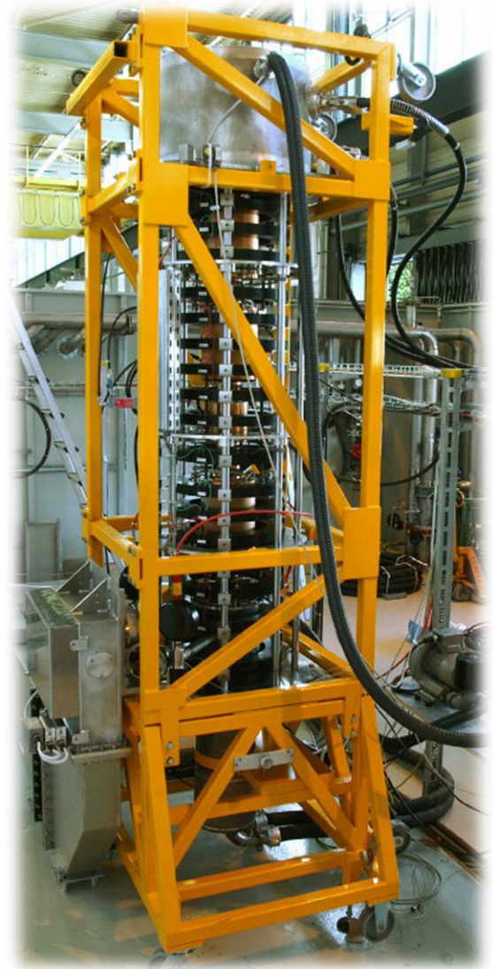
CERN LHC: 400 MHz, 300 kW, CW, \eta 62 %
