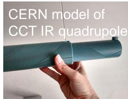
CERN model of CCT IR quadrupole
