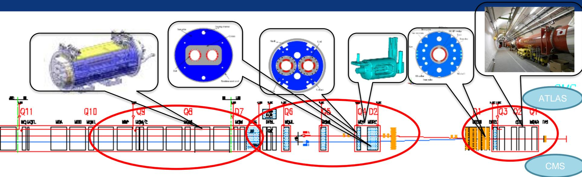
3. For collimation we also need to change the DS in the continuous cryostat:
