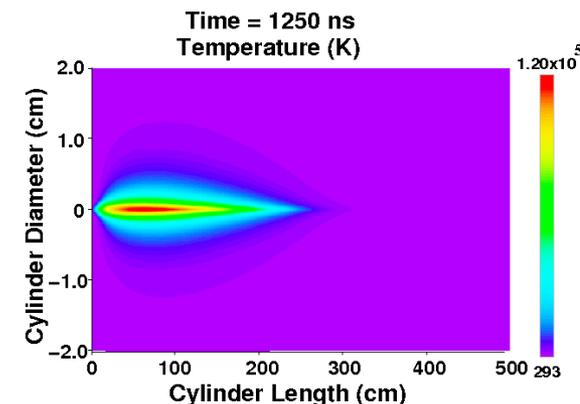
Huge energy to be extracted and dumped => need large dump section
