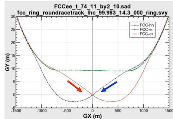
Max. separation of 3(4) rings is about 12 m: wider tunnel or two tunnels are necessary around the IPs, for  $\pm 1.2$  km.
