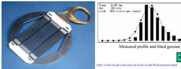
SEM grid with 15 foils to measure the beam profile. The large foils at either side of the grid are connected electrically together to form a 16-th channel.
