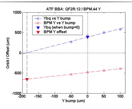
Beam-based alignment in the KEK-ATF damping ring:
