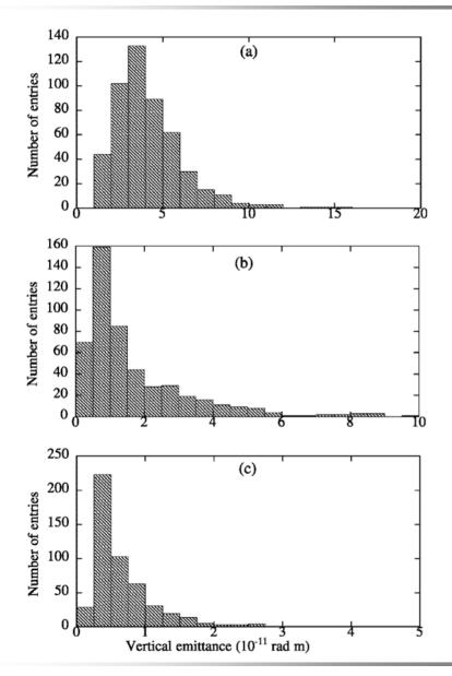
Simulations of emittance tuning in the ATF damping ring.
