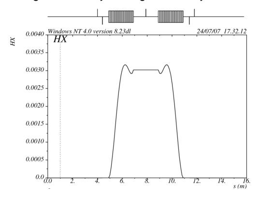
Note that we use the same dipoles (bending radius and length) for our example in both cases (FODO and DBA). In the DBA lattice the curly-H function is reduced by a significant factor, compared to the FODO lattice.
