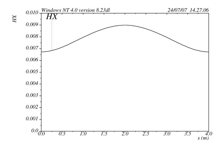
As a first attempt at reducing the natural emittance, let us try designing a lattice that has zero dispersion at one end of each dipole. This can be achieved using a double bend achromat (DBA) lattice.
