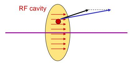
Fortunately, RF cavities are usually designed with a longitudinal electric field, so that particles experience a change in longitudinal momentum as they pass through, without any change in transverse momentum.
