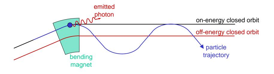
By considering the change in the phase-space variables when a particle emits radiation carrying momentum dp, we find that the associated change in the betatron action is:
