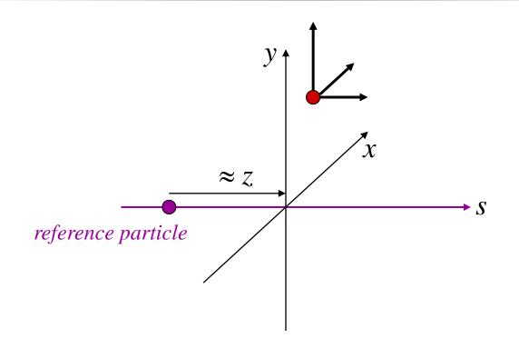
The reference particle is a particle travelling along the reference trajectory with momentum  $P_0$  and velocity  $\beta_0 c$ .
