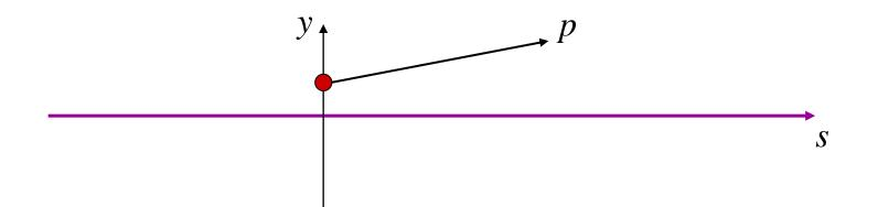
A relativistic particle will emit radiation with an opening angle of  $1/\gamma$  with respect to its instantaneous direction of motion, where  $\gamma$  is the relativistic factor.
